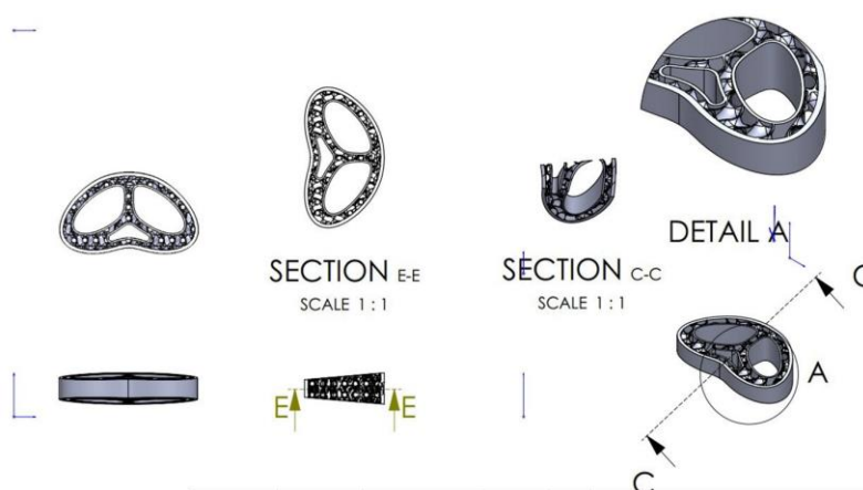
Figure 2. Industrial map of lumbar cage design 1 with a gyroid porous structure
